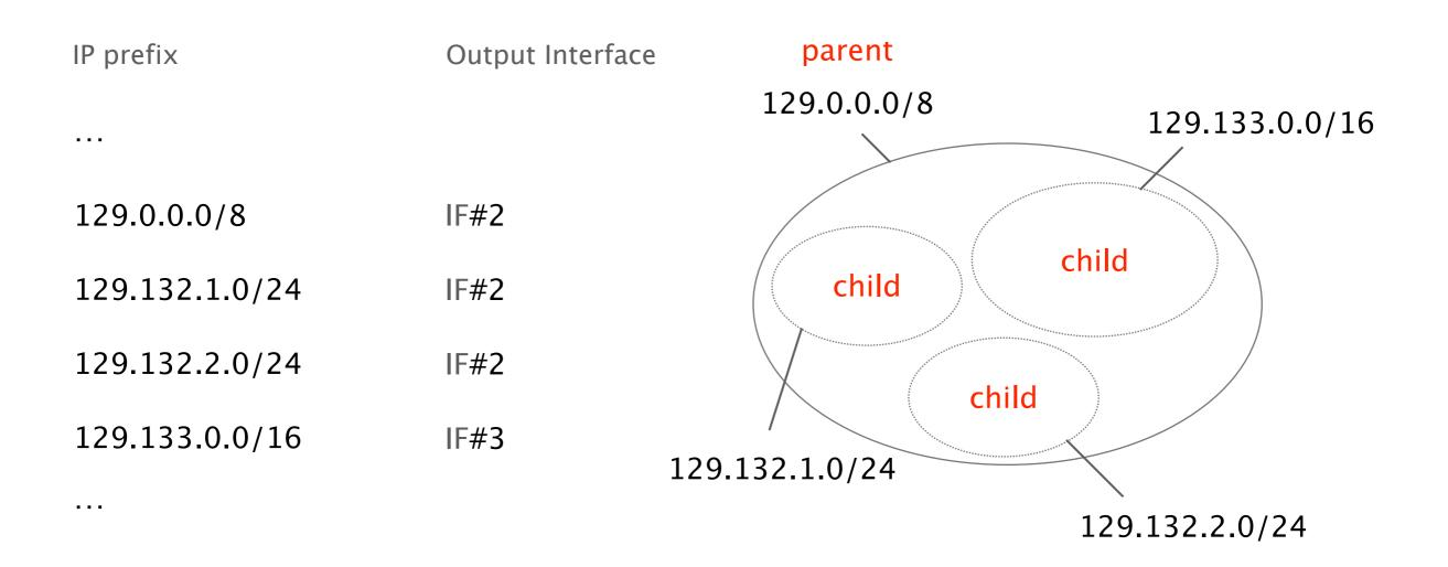
Forwarding is done along the most specific prefix, *i.e.*, the smallest set containing the IP address
